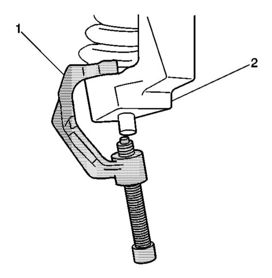
Fig. 16: Lower Ball Joint & Steering Knuckle Courtesy of GENERAL MOTORS CORP.
