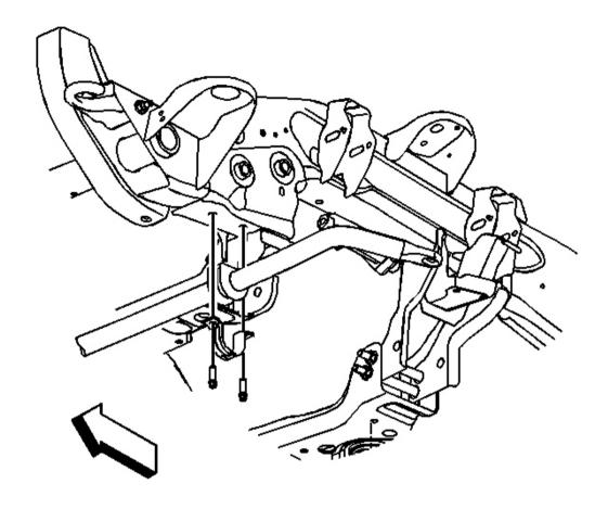
Fig. 4: Insulators & Stabilizer Shaft Courtesy of GENERAL MOTORS CORP.
