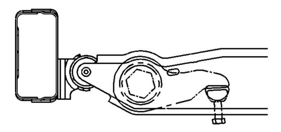
Fig. 30: Turning Adjustment Bolt Clockwise Or Counterclockwise Courtesy of GENERAL MOTORS CORP.
