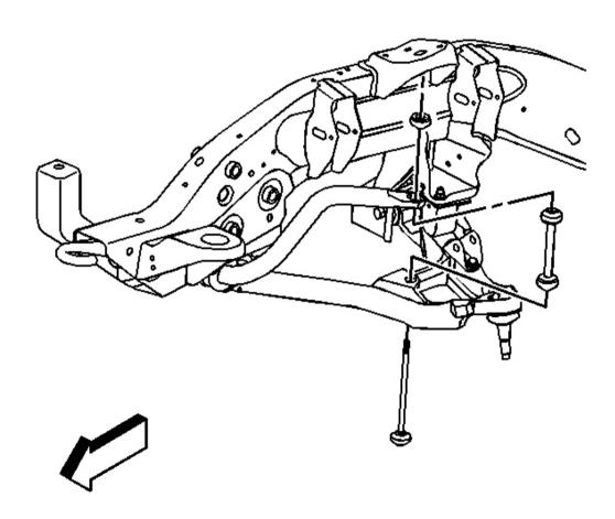
Fig. 7: Link Bolts & Link Assemblies Courtesy of GENERAL MOTORS CORP.
