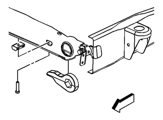
Fig. 29: Adjustment Bolt & Adjuster Nut Courtesy of GENERAL MOTORS CORP.
