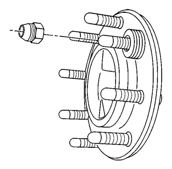
Fig. 21: Installing The New Stud Into The Hub Flange Hole Courtesy of GENERAL MOTORS CORP.
