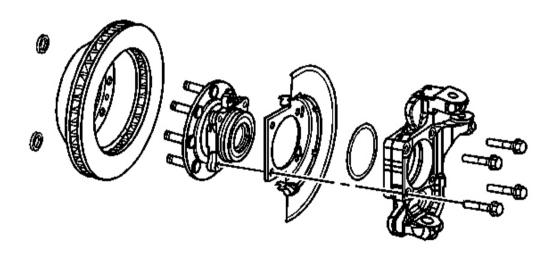
Fig. 23: O-Ring & Steering Knuckle Courtesy of GENERAL MOTORS CORP.
