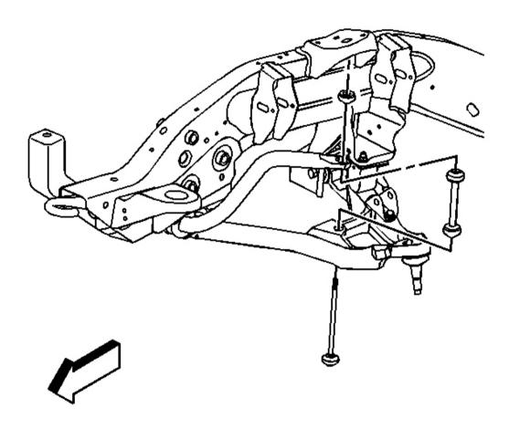
Fig. 5: Link Bolts & Link Assemblies Courtesy of GENERAL MOTORS CORP.
