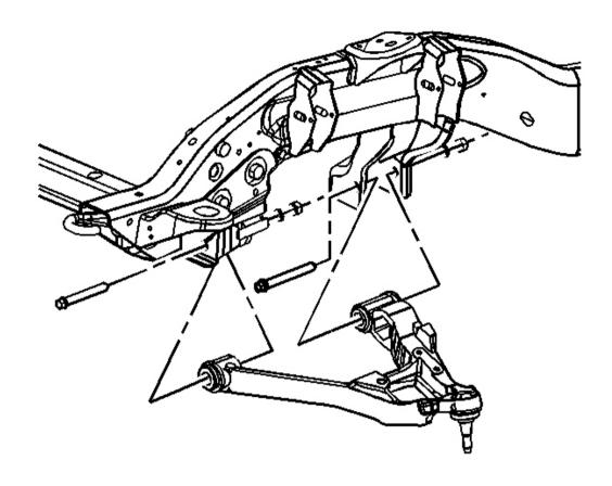
Fig. 17: Lower Control Arm Bolts
