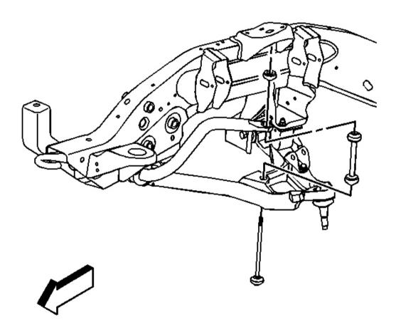
Fig. 6: Link Bolts & Link Assemblies Courtesy of GENERAL MOTORS CORP.
