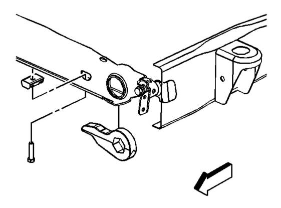
Fig. 25: Adjustment Bolt & Adjuster Nut Courtesy of GENERAL MOTORS CORP.
