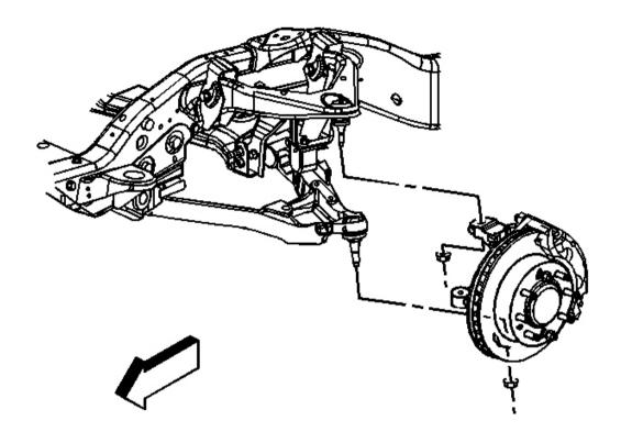
Fig. 13: Identifying Steering Knuckle Courtesy of GENERAL MOTORS CORP.
