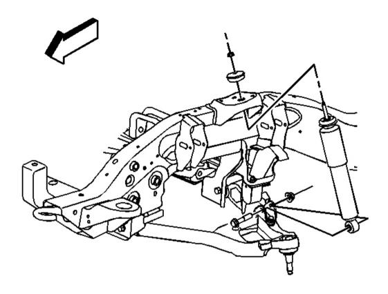
Fig. 31: Shock Absorber & Tennon End Courtesy of GENERAL MOTORS CORP.
