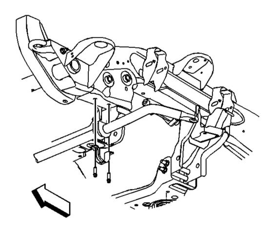
Fig. 8: Insulators & Stabilizer Shaft Courtesy of GENERAL MOTORS CORP.
