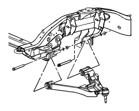
Fig. 18: Lower Control Arm Bolts
