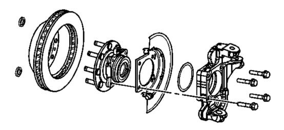
Fig. 22: O-Ring & Steering Knuckle Courtesy of GENERAL MOTORS CORP.
