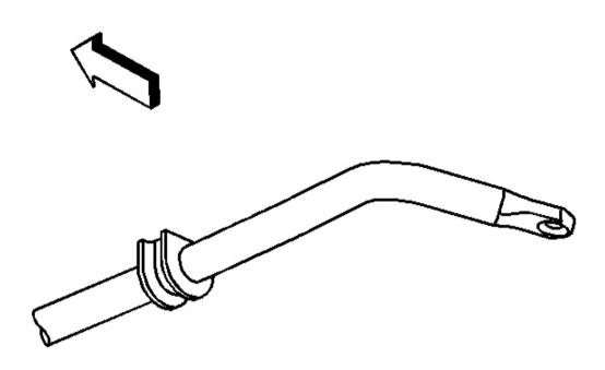
Fig. 9: Placing Insulators On Stabilizer Shaft Courtesy of GENERAL MOTORS CORP.
