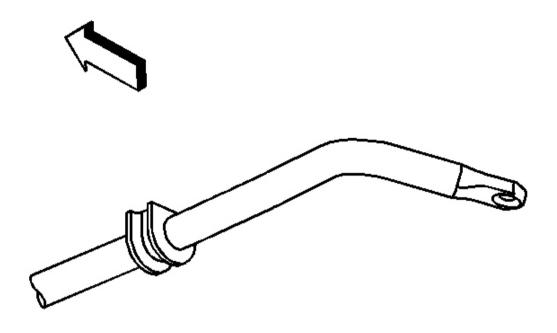
Fig. 3: Placing Insulators On Stabilizer Shaft Courtesy of GENERAL MOTORS CORP.
