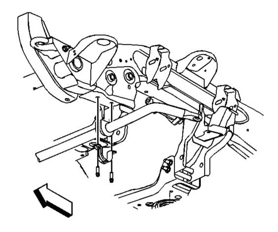
Fig. 10: Insulators & Stabilizer Shaft Courtesy of GENERAL MOTORS CORP.
