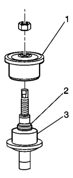
Fig. 36: Identifying Upper Insulator Courtesy of GENERAL MOTORS CORP.
