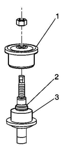
Fig. 32: Identifying Upper Insulator Courtesy of GENERAL MOTORS CORP.
