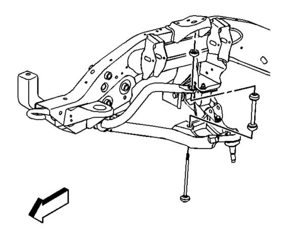
Fig. 1: Link Bolts & Link Assemblies Courtesy of GENERAL MOTORS CORP.
