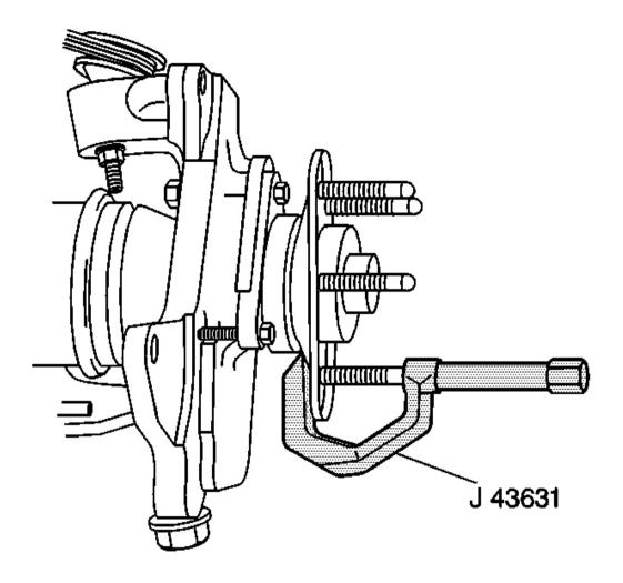
Fig. 20: Removing Wheel Stud From Hub Flange Courtesy of GENERAL MOTORS CORP.
