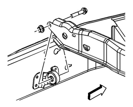
Fig. 27: Torsion Bar Crossmember Courtesy of GENERAL MOTORS CORP.
