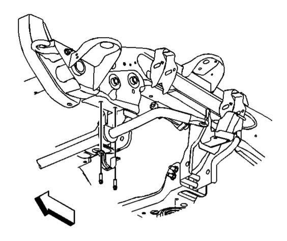
Fig. 2: Insulators & Stabilizer Shaft Courtesy of GENERAL MOTORS CORP.
