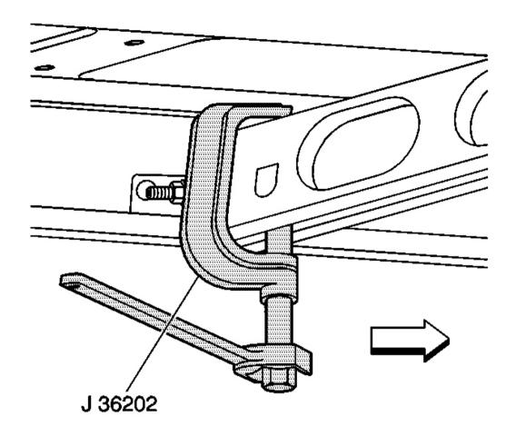
Fig. 28: Installing J 36202 To Adjustment Arm & Crossmember Courtesy of GENERAL MOTORS CORP.
