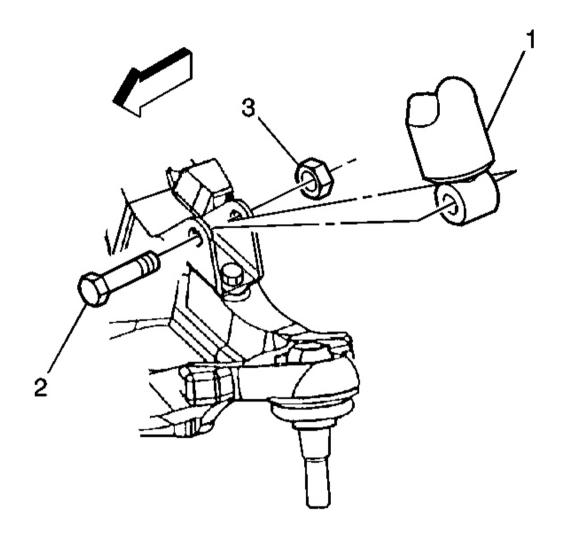
Fig. 33: View Of Shock Absorber Courtesy of GENERAL MOTORS CORP.
