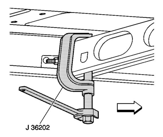
Fig. 24: Installing J 36202 To Adjustment Arm & Crossmember Courtesy of GENERAL MOTORS CORP.
