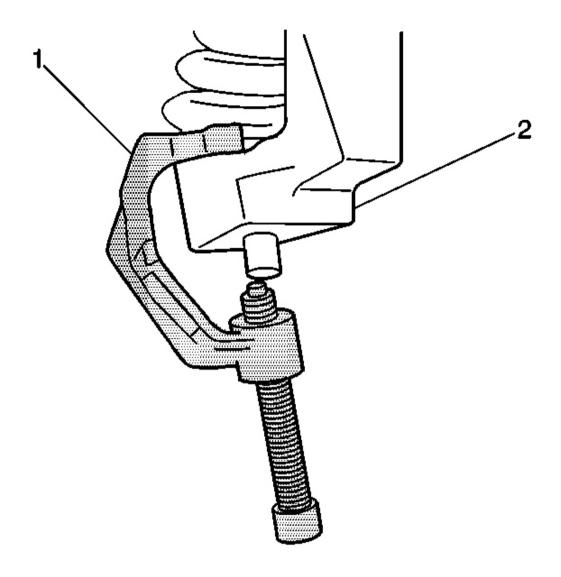
Fig. 11: Lower Ball Joint & Steering Knuckle Courtesy of GENERAL MOTORS CORP.
