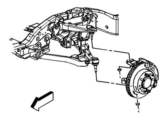
Fig. 12: Identifying Steering Knuckle Courtesy of GENERAL MOTORS CORP.
